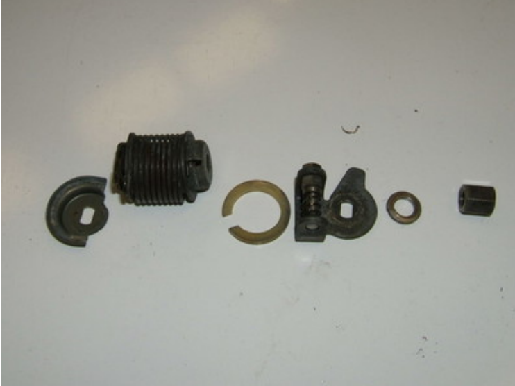
RH stock throttle body with linkage disassembled. NOTE: Some newer style Z32 RH throttle bodies have the stop (pictured here to the left hand side of the pic) located on the inside of the throttle body instead of the outside like pictured here. The Z1 Upgraded throttle bodies are made to accomodate either style stop:
