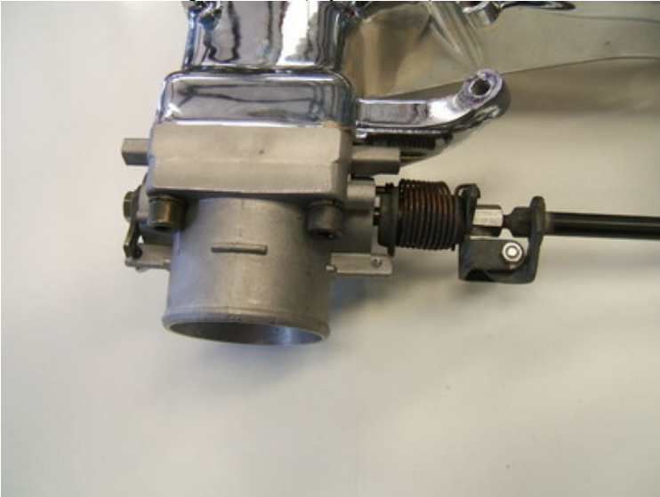
RH Z1 Throttle Body installed:
