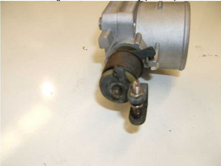
Assembling end of linkage onto Z1 LH throttle body:
