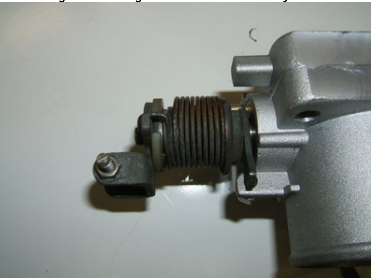
Assembling end of linkage onto Z1 LH throttle body:
