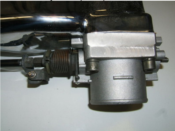
LH Z1 Throttle Body installed (top view):
