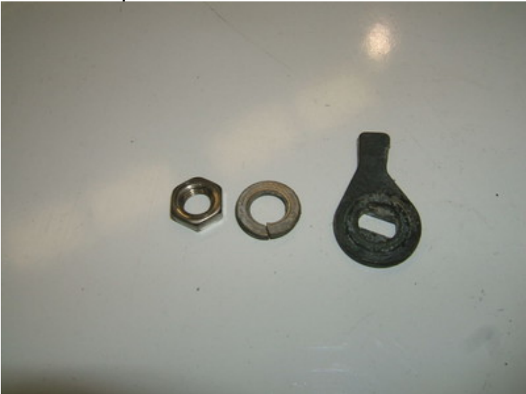
Throttle body linkage from RH throttle body (early style) Newer models will also have the stop which would be located on the left side of the pic:
