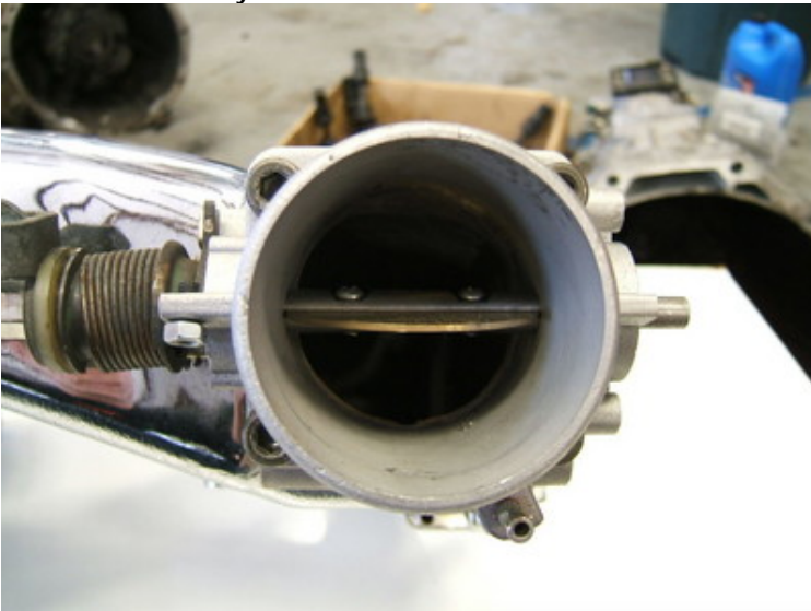
Inside of Z1 Throttle Body with plenum ground down and port matched.:
