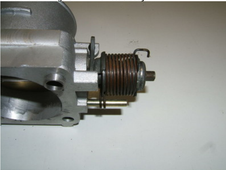
Most of the linkage on Z1 LH throttle body:
