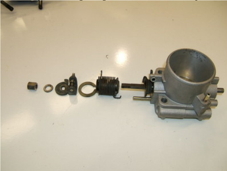
Linkage spread out and ready to be placed on to Z1 LH throttle body:
