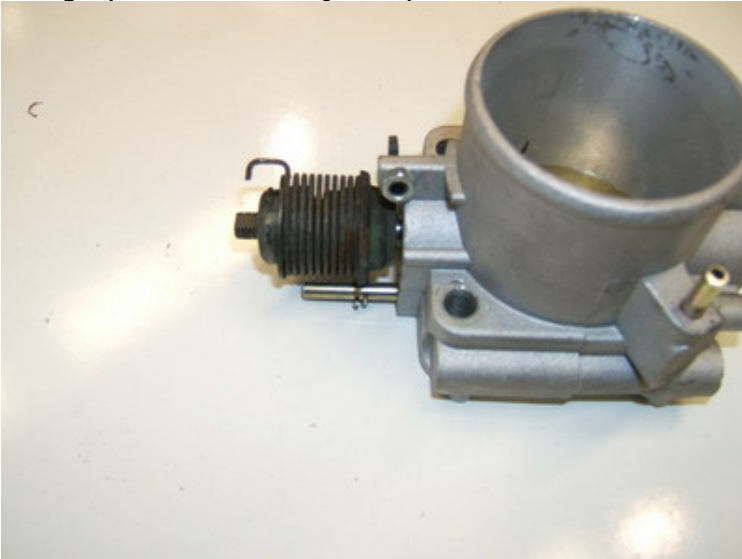
Most of the linkage on Z1 LH throttle body:
