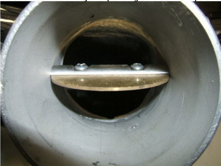
Inside of Z1 Throttle Body with plenum ground down and port matched.:
